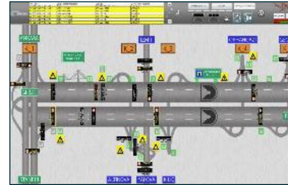
Tunnel SCADA System
